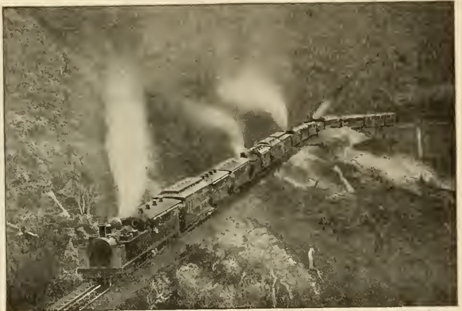
AN EXCURSION TRAIN DRAWN BY FOUR FELL ENGINES ON THE RIMUTAKA INCLINE. GRADE, 1 IN 15; WEIGHT OF TRAIN, 174 TONS; LENGTH OF TRAIN, 648 FEET.
